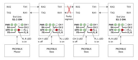
If an optical fibre segment fails, all communication with units beyond the faulty fibre segment will be lost. To determine witch fibre segment has failed, look at the FL L, CH 1 and CH 2 LED's as show in the picture above.
