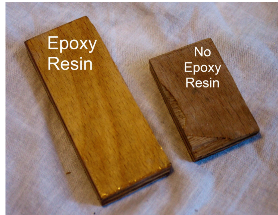
Figure 5: The epoxy treated wood shows little sign of degradation, while the non-treated control piece has become discoloured and has had pieces fall off around the edge upon handling after the experiment, suggesting fragility.
