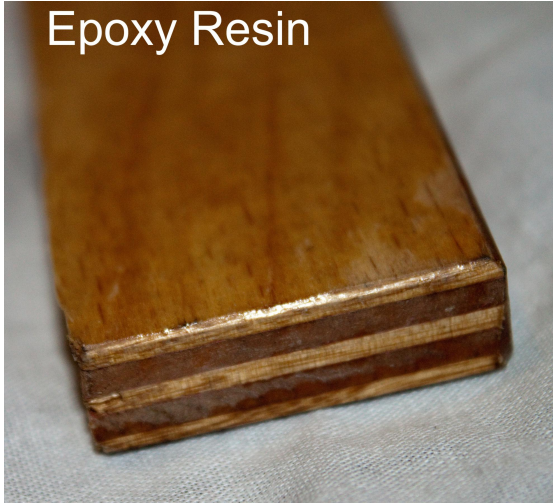
Figure 7: The epoxy coating appears to have kept water out of the wood, leaving it in a better condition after weathering.
