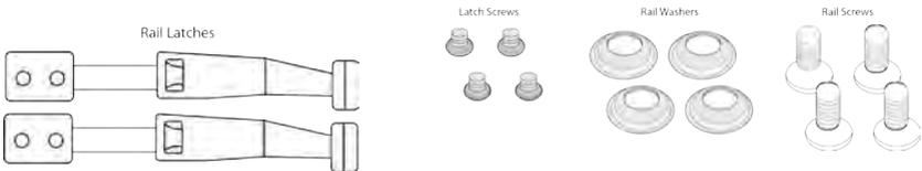
1. On the right and left sides of the FileCruiser Server 1U4, secure the Rail Latches to the FileCruiser Server 1U4 housing using the latch screws, two screws for each latch.
