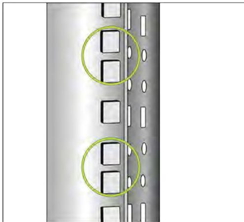
3. Secure the rails to the rack posts. Make sure the rack rails are properly oriented in the rack.
