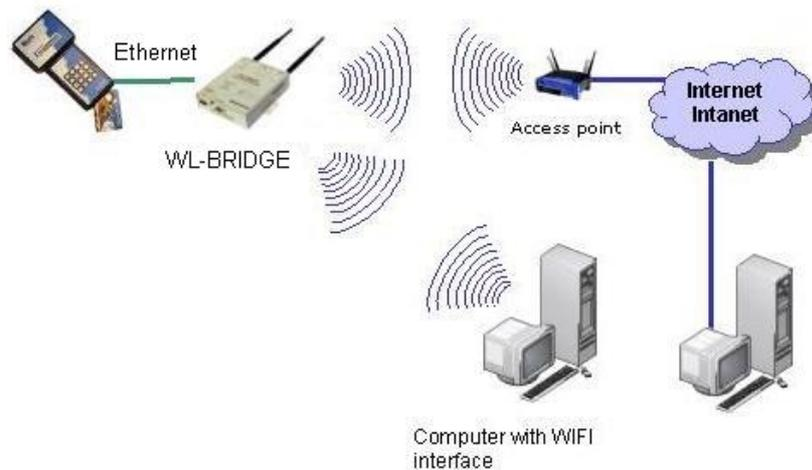
In infrastructure mode, you must have an Access Point (AP) in your application. In this mode, WL-BRIDGE can communicate with all devices on your wired network and all devices on your WIFI network through AP.
