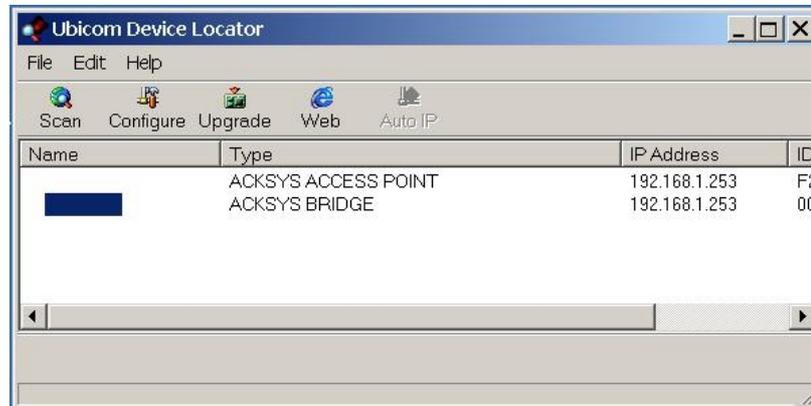
Locator scans your network to locate all WL-BRIDGE, If your WL-BRIDGE is not ready (turn on, and connected on your computer), click on scan button when it is ready.
