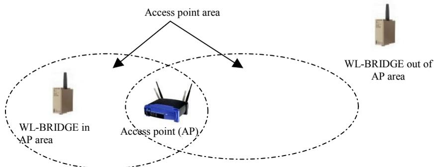
If WL-BRIDGE is out of the AP area, all RF signal quality LEDs blink. If WL-BRIDGE is in the AP area, you can see RF Signal quality reception on the LEDs.
