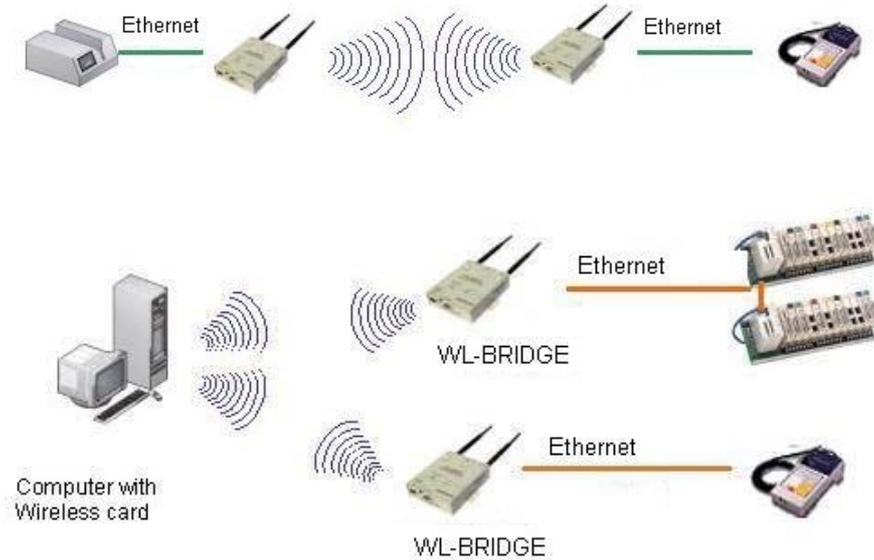
In AD-HOC mode, WL-BRIDGE can establish directly a communication with an other WIFI equipment. This equipment can be an other WL-BRIDGE or a device with WIFI interface. In this mode, WL-BRIDGE can't communicate with an Ethernet 10/100 BT interface equipment.
