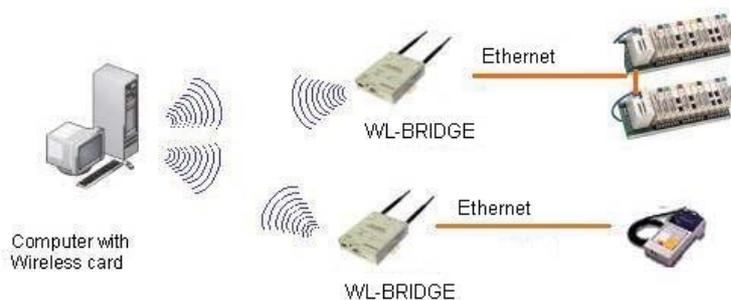
In AD-HOC mode, you must have the same SSID and channel in all devices. If WL-BRIDGE don't have the same channel, you can't communicate with it.
