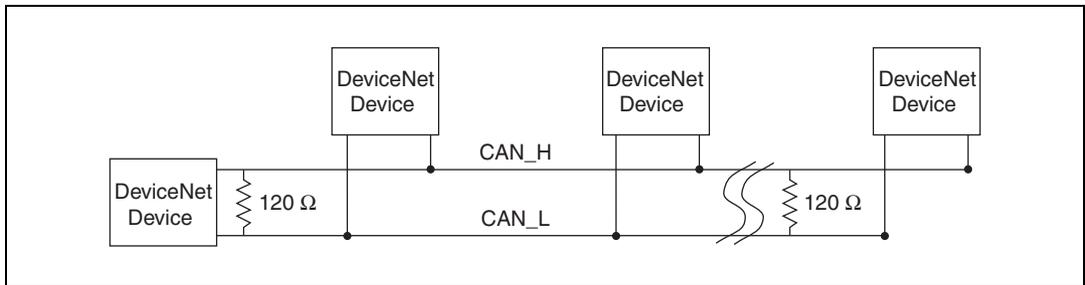
**Figure B-7.** Termination Resistor Placement
