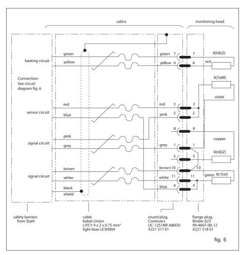
• Install equipotential bonding along the complete cable run of the intrinsically safe circuit from the monitoring head to the grounding system near the flow meter.
