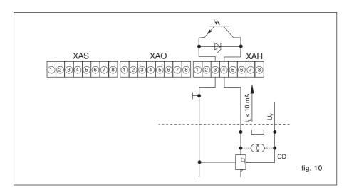
The FC01-Ex driver output comprises an integral safety circuit which when releasing the counter operating coil will limit overvoltages caused by inductance and convert the energy stored.
