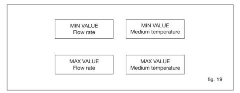
After switch-on or NOT-BUSY indication, the minimum and maximum values are deleted and will be continuously updated (non-return pointer principle).
