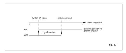
With limit switch 1 set for flow rate and a flow volume/time unit selected in menu DISPLAY
