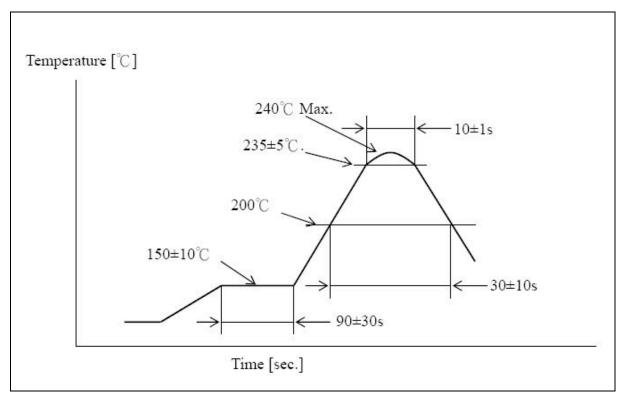
Pre heating temperature:  $150\pm10[^{\circ}\mathbb{C}]$  Pre heating time:  $90\pm30[\sec.]$  Heating temperature:  $235\pm5[^{\circ}\mathbb{C}]$  Heating time:  $10\pm1[\sec.]$
