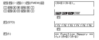
If the function memory number you assign a function to already contains a function, the previous function is replaced with the new one.
