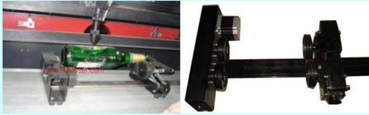
Rotary Attachment with rollers--it can engrave on the material like bottles or cups.
