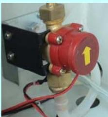
The laser machine can be equipped with a chiller or water pump and tank. In either case, the coolant must keep the laser tube from over heating. This check sensor ensures the laser will not be allowed to fire without proper coolant flow. It is typical for us to use a mixture of glycol (or Antifreeze) and water as the coolant fluid.
