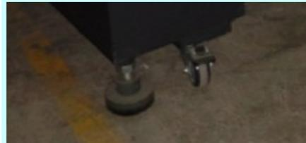
WISELY various models of laser engraving & cutting machines can weigh from 100 kg to more than 1200 kg. Every machine is equipped with castor wheels to make it easier to move it around the workshop or office.
