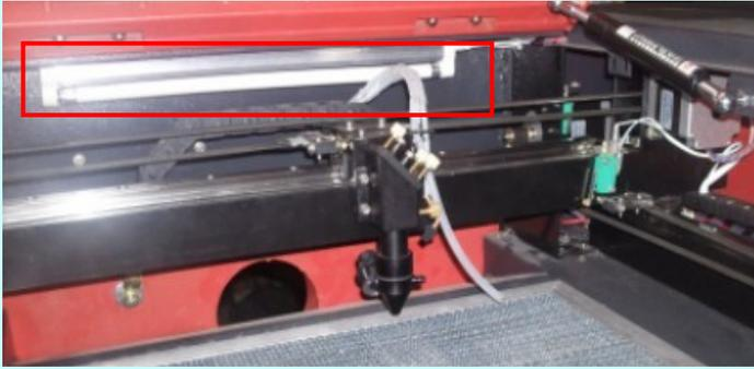
It is always nice to check on the progress of the project that is currently running. The laser machine has a viewing window through the main access door, and this interior light works great for providing enough light to see what is happening inside.
