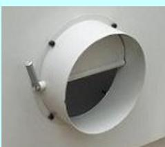
The air that exits the laser machine can be controlled by this vent damper. It allows the operator to select what proportion of air can be pulled from above or below the work surface.
