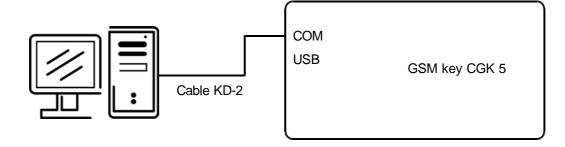
• cable KD2 is connected to PC serial port (example COM1)
