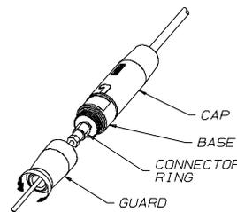
Figure 2-23. Attaching Probe to Sample Line
