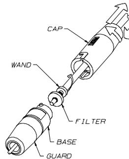
Figure 2-24. Changing the Probe Filter
