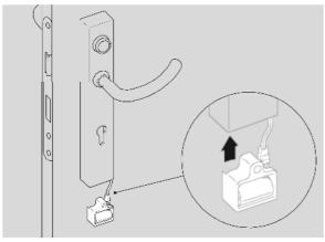
Abb. 6: Insert battery holder
