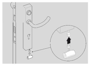
Fig. 5: Connect battery
