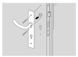
Push the interior fitting onto the door leaf and attach it with the upper screws (short).
