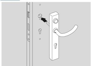
Push the exterior fitting into the appropriately prepared door leaf.
