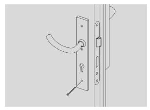
8. Insert the lower screw (long) and fasten the battery holder in place.
