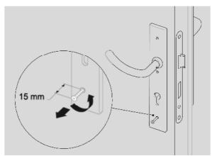
Fig. 8: Remove battery holder
