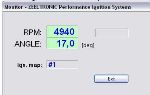
⇒ Monitor show engine revolution, ignition advance angle, selected ignition map, rev limit activation.
