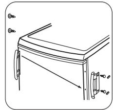
12. Remove and install the handle<sup>1)</sup> on the opposite side.
