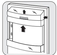
Gradually pull the shelf in the direction of the arrows until it comes free, then reposition as required.
