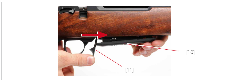
Fig.12 Sliding the magazine holder forwards
