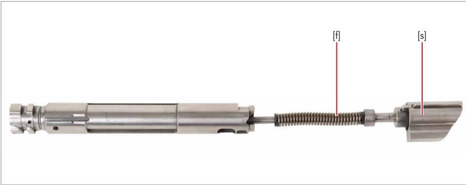
Fig. 23 Withdrawing the firing pin and spring
