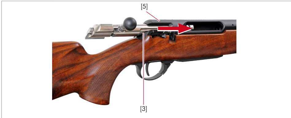
Fig.20 Inserting the bolt
