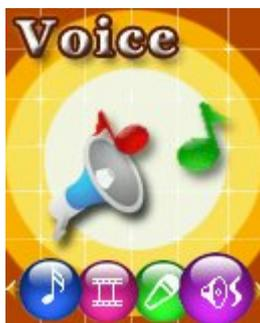
Use “◀◀” and “▶▶” to navigate through the main menu. Select Voice and press “M” to enter. The Voice menu allows you to replay the recorded files.
