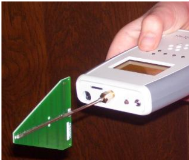
Measurement position with LogPer antenna
