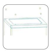
2. Unscrew and lift the lid from the rear and remove it, them lift the upper door and replace it on a padded surface to prevent it scratched.
