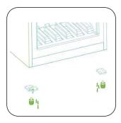
7. Unscrew and remove the bottom hinge pin, turn the bracket over and replace it. Refit the bracket fitting the bottom hinge pin. Replace both adjustable feet. Transfer the lower door to the opposite position. Secure the door's level, make the bottom hinge pin into the lower hole of the door, then tight the bolts.
