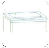
3. Remove the upper hinge core, transfer it to left side and tighten securely, then put it in a safe place.
