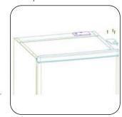
4. Remove the two flange screw, then remove the middle hinge that hold the lower door in place. Lift the lower door and place it on a padded surface to prevent scratching it.
