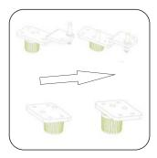
8. Make the middle hinge reverse the direction 180°, then transfer it to the left property position. Make the middle hinge pin in the upper hole of the lower door, then tight the bolts. Transfer the lower door to the opposite position. Secure the door's level; make the middle hinge pin into the lower hole of the upper door
