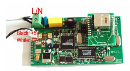
The AC or DC powerline line can be connected to the L/N connector denoted on the above picture.
