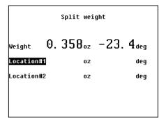
For instance we have a fan with the blades difference 15 deg. It means we can install mass to the position 0 deg,  $\pm$  15 deg,  $\pm$  30 deg,  $\pm$  45 deg, ... Required position lies between -15 deg and -30 deg. We enter these values to split weight screen. After both angles definitions the result masses are calculated.
