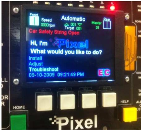
Pixel home screen displays **Car Safety String Open** Fault (shown in red).
