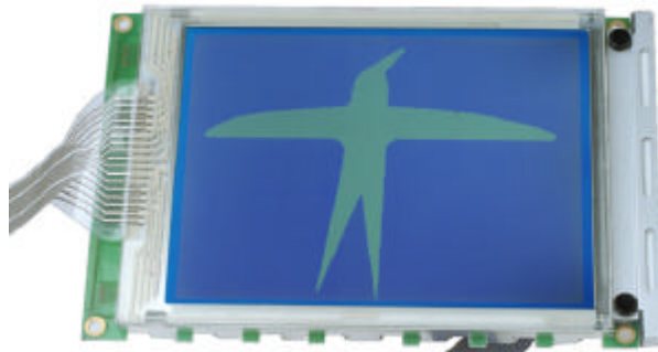
Figure 1.2 Front view of the SmartLCD: 320x240 graphic LCD displaying bird
