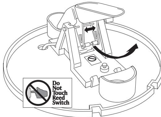
4. Separate an end cap from one side of the magnet.
