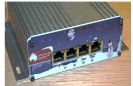
4 DMX universe E1.31 to DMX Protocol Bridge
