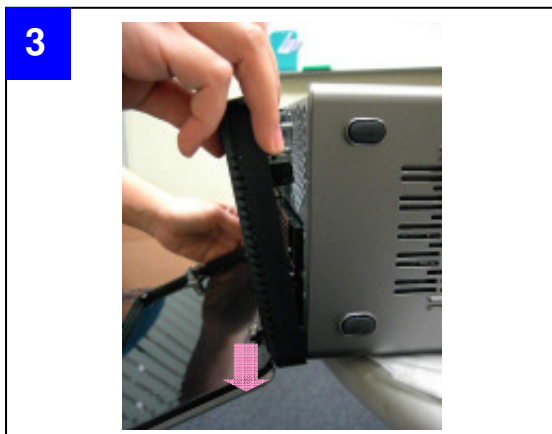
■ Angle the latch until it is 15 degree away from the chassis
