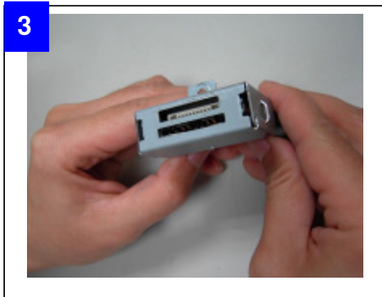
■ Remove the seal on the holder and make sure the sockets is right to the opening
