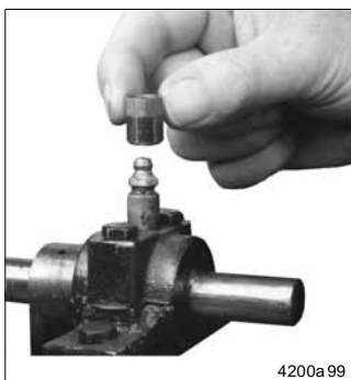
Fig. 2-1 Place the Zerk-Lock body over the grease nipple
