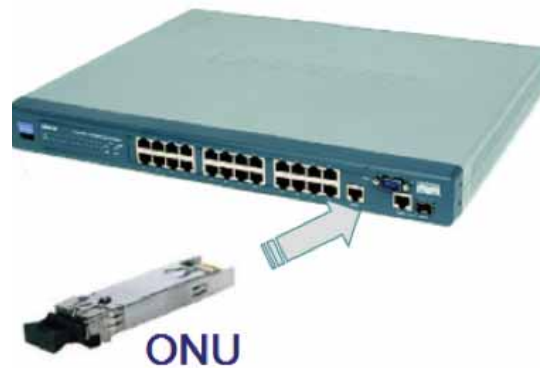
Figure 8. SFP ONU lets operators use their current Ethernet edge switches when deploying a POL.
