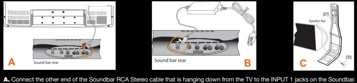
C. See the documentation that came with the Soundbar to connect other audio devices to the Soundbar. Reattach the Soundbar to the brackets using the wing screws [33]. Note: If the Soundbar is not level with the TV, slightly unscrew the screws [29 & 32] using the wrench [14] then reposition the Soundbar and re-tighten
