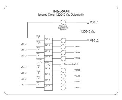
**Note** — The output circuits are electrically isolated from each other (the commons are NOT connected internally). Therefore, up to eight different voltage sources (VS0–VS7) may be used.
