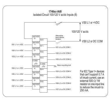
Note — The input circuits are electrically isolated from each other (the commons are NOT connected internally). Therefore, up to eight different voltage sources (VS0–VS7) may be used.
