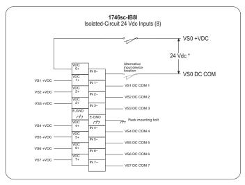
$\begin{tabular}{ll} \textbf{Note} & -- \text{The input circuits are electrically isolated from each other (the commons are NOT connected internally). Therefore, up to eight different voltage sources (VS0-VS7) may be used. \\ \end{tabular}$
