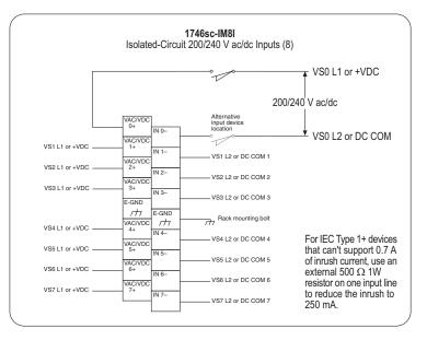
Note — The input circuits are electrically isolated from each other (the commons are NOT connected internally). Therefore, up to eight different voltage sources (VS0–VS7) may be used.
