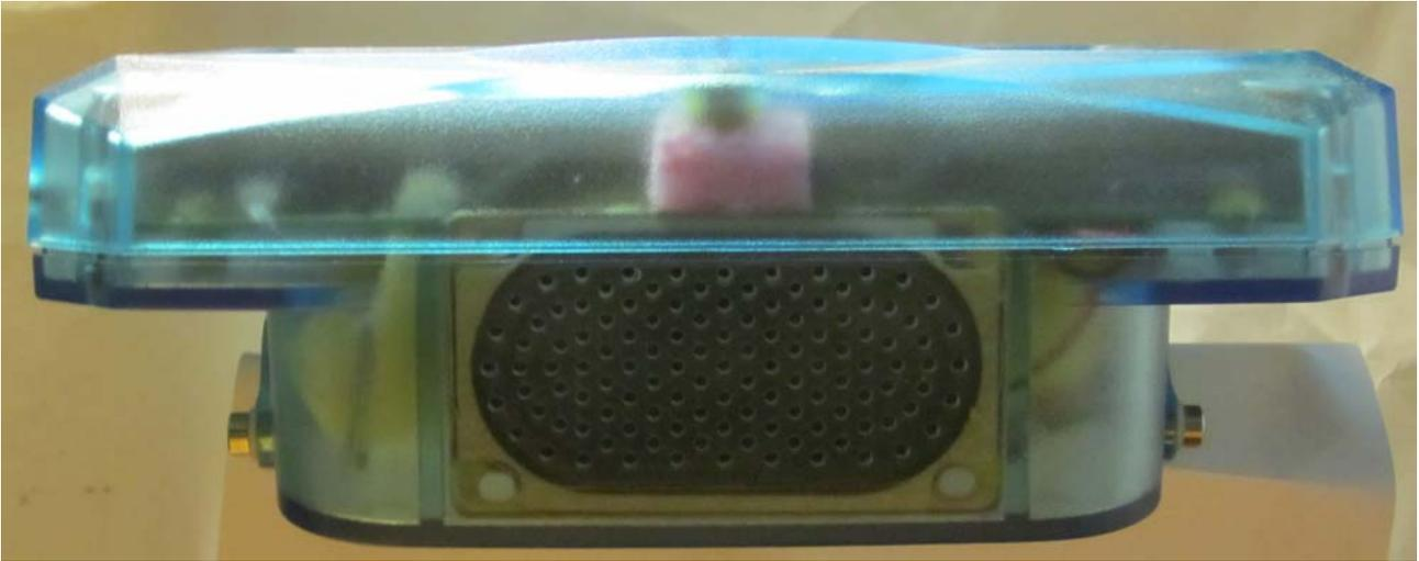
**Front view - A large oval speaker is mounted directly below the screen. Facing out, it is never muzzled when the device is placed flat on a table. This is probably the biggest speaker you will find in an Augmentative Communication Aid!**
