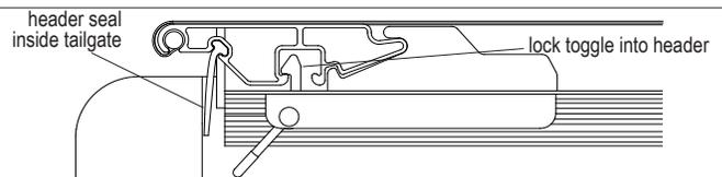
**STEP 8:** To release cover, Trigger pull rear release toggle. Start rolling cover toward cab making sure both sides of cover roll evenly. For best results leave unrolled portion of cover attached to the hook fastener and Velcro® loop fasteners while opening.
