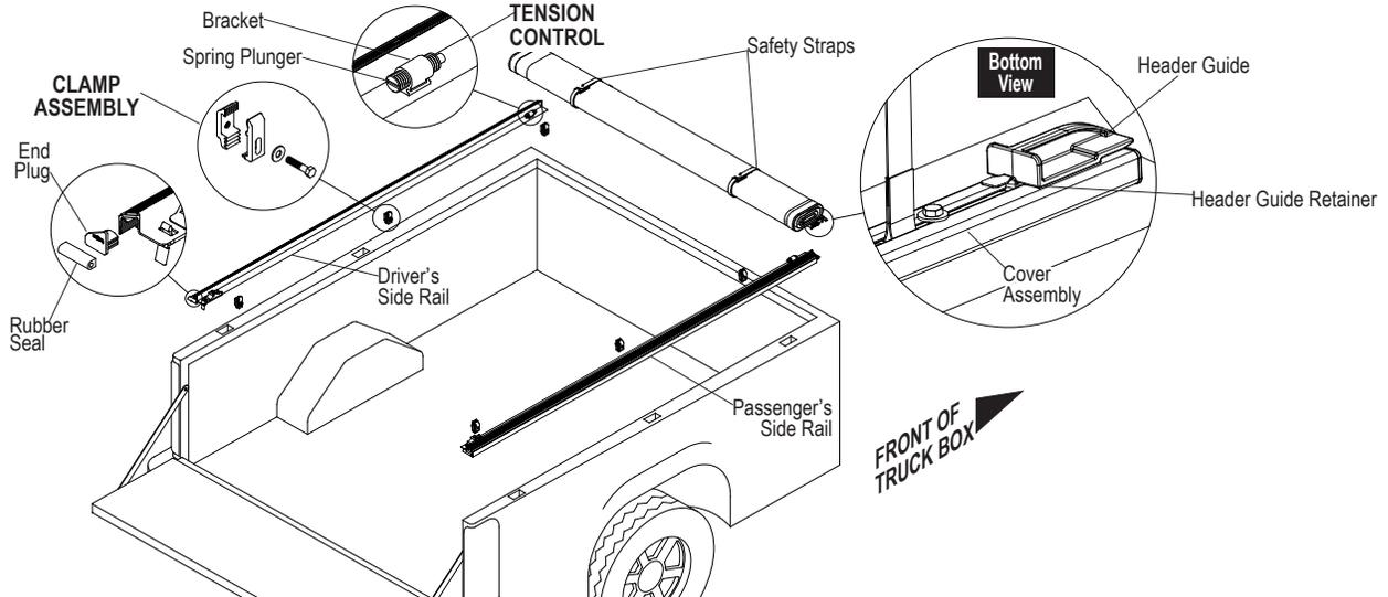
**STEP 1:** Attach the TruXedo rails to the truck's vertical inside flange as shown in Detail A. To get the correct TruXedo rail alignment from front to back, see Detail-B. Compress the rear D-seal against the closed tailgate and hold. Attach clamps starting at the tailgate. Evenly space 3 clamps along each TruXedo rail, leaving approximately 8" on each end.
