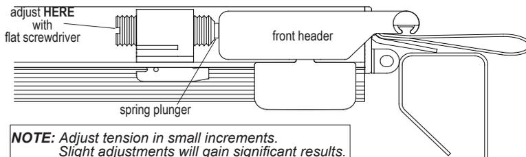
**NOTE:** Adjust tension in small increments. Slight adjustments will gain significant results.
