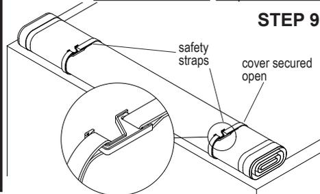
**STEP 9:** Secure cover open by hooking safety straps to front loops.
