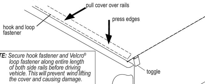
**NOTE:** Secure hook fastener and Velcro® loop fastener along entire length of both side rails before driving vehicle. This will prevent wind lifting the cover and causing damage.
