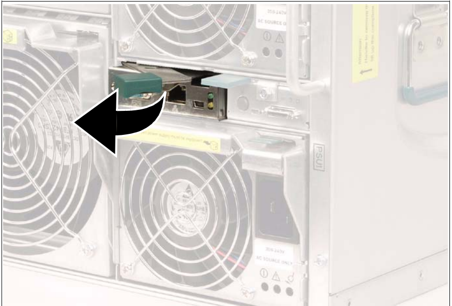
Figure 63: Disengaging the management blade
