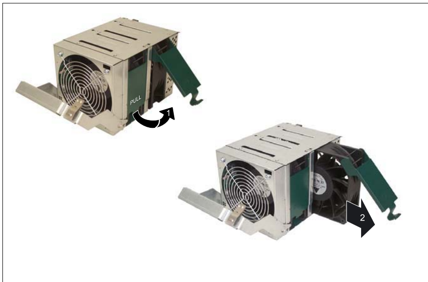
Figure 85: Disengaging the fan unit (a = green touch point)
