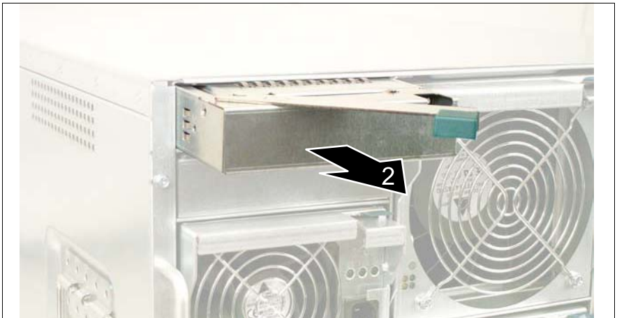
Figure 47: Removing the dummy module
