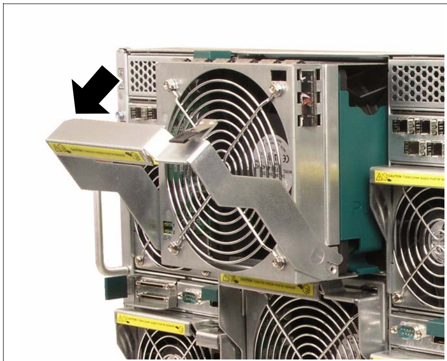
Figure 84: Removing the fan unit
