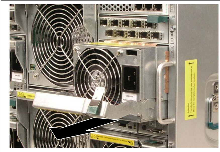
Figure 79: Removing the PSU
