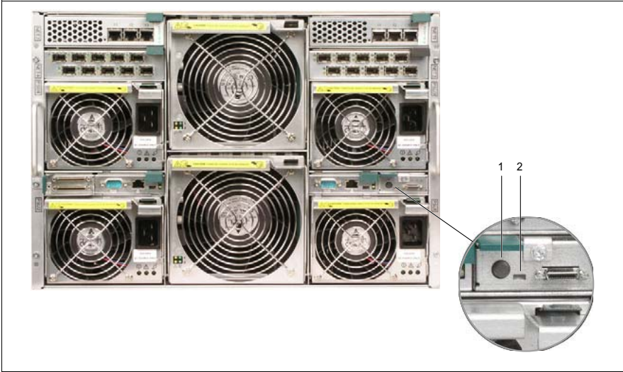
Figure 15: System operating and indicator elements on the rear
