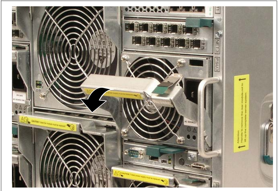
Figure 78: Removing the power supply unit
