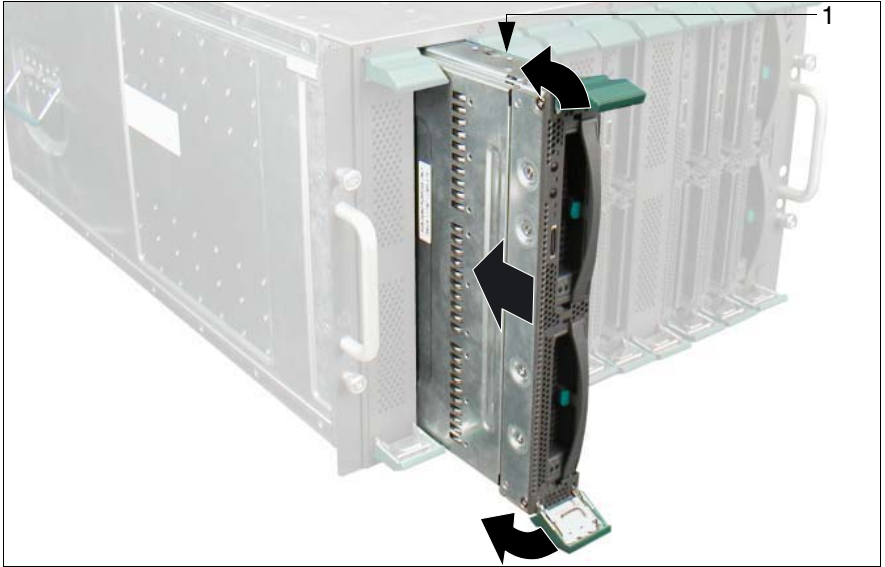
Figure 32: Inserting the server blade
