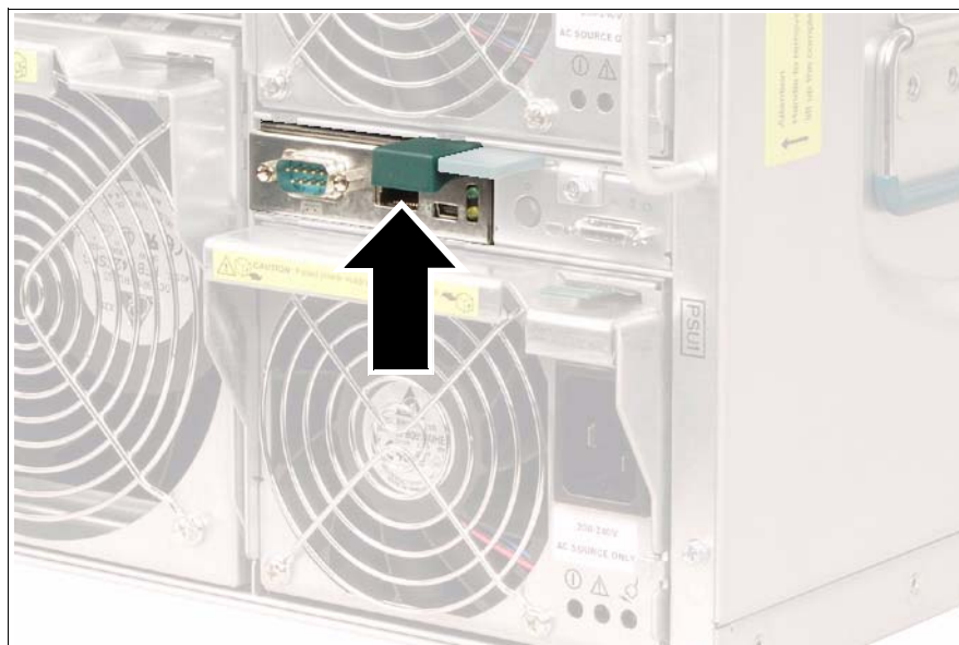
Figure 62: Disengaging the management blade
