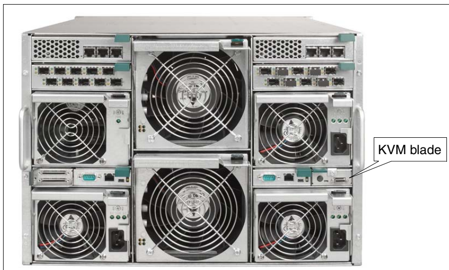
Figure 65: Position of the KVM blade
