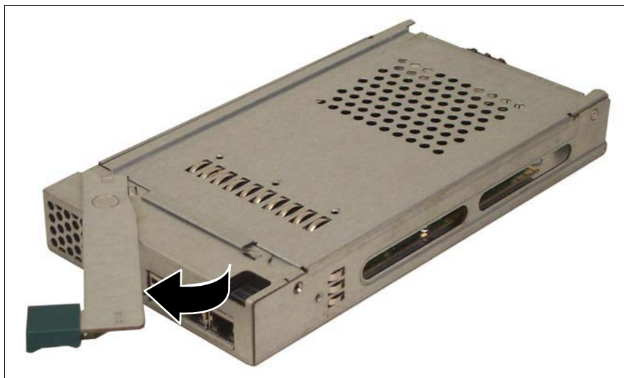
Figure 48: Disengaging the I/O blade
