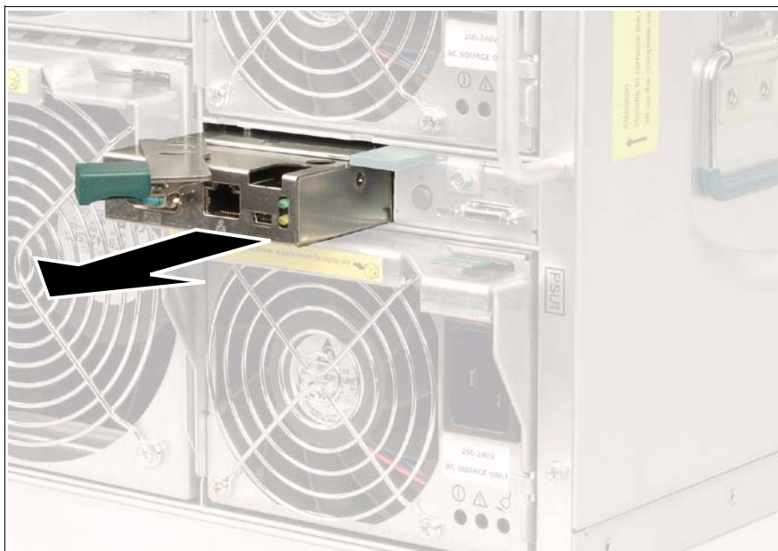
Figure 64: Removing the management blade
