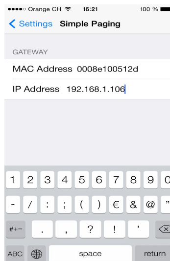
Illustration 3: By defining a particular Gateway, the App locks to it on startup
