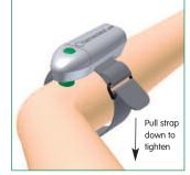
The unit can now be secured by folding the Velcro strap back on itself and attaching the end of the strap onto the fibrous surface.
