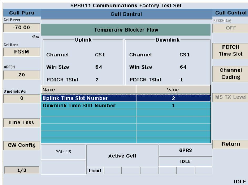
Figure 1-19 PDTCH Time Slot parameter setting interface
