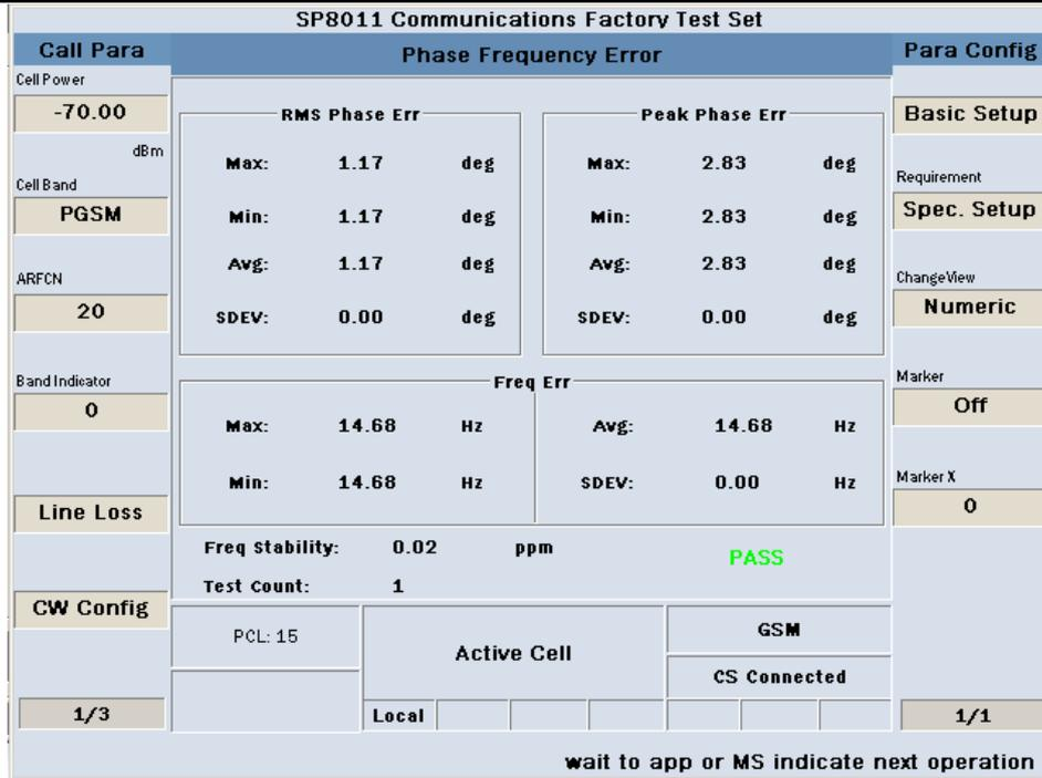
Figure 2-5 the phase frequency error testing results in data
