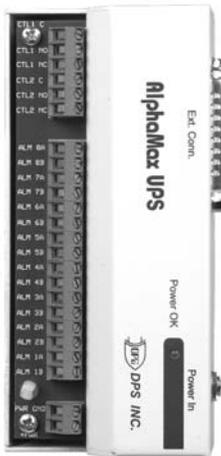
The Connector block mounts on any flat surface near the AlphaMax. A 3-foot cable is included for interfacing the AlphaMax. All alarm and control points connect at the wire wrap posts or screw lug terminals on the connector, making installation quick and clean. No soldering is required.
