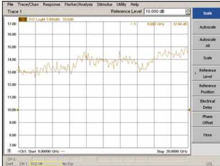
Figure 2-3 RF Output Gain with +2 dBm ALC Off
