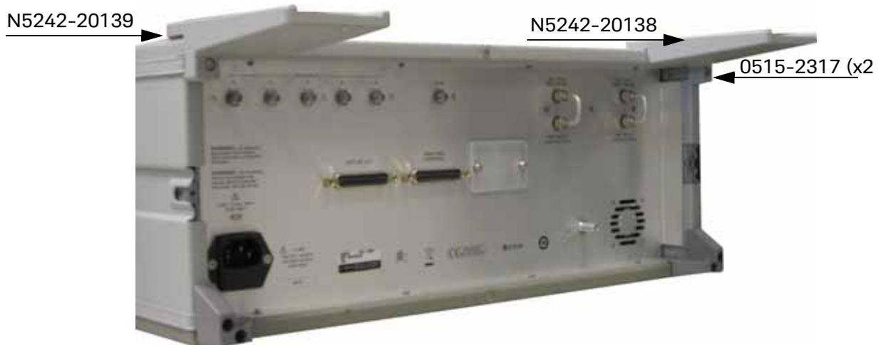
6. Place the analyzer on top of the test set and ensure that the front frame of the analyzer is positioned slightly forward of the locks that are attached to the test set. Slide the analyzer back so the locks engage the front frame of the analyzer.
