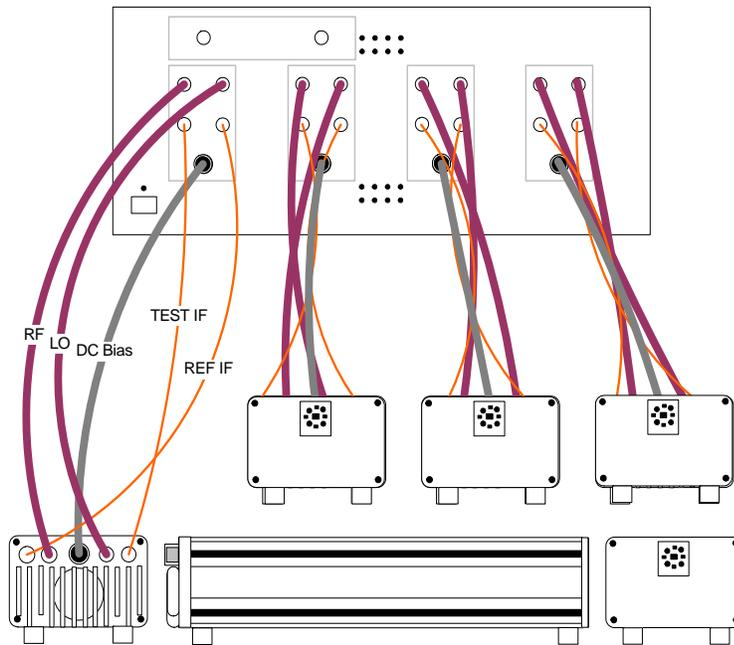
Figure 1-24 Example; VDI Module Connections
