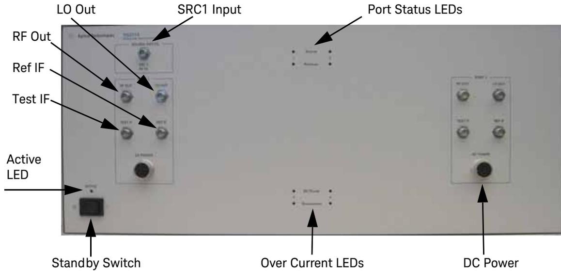
Figure 1-6 N5262A (4-Port) Front Panel Features
