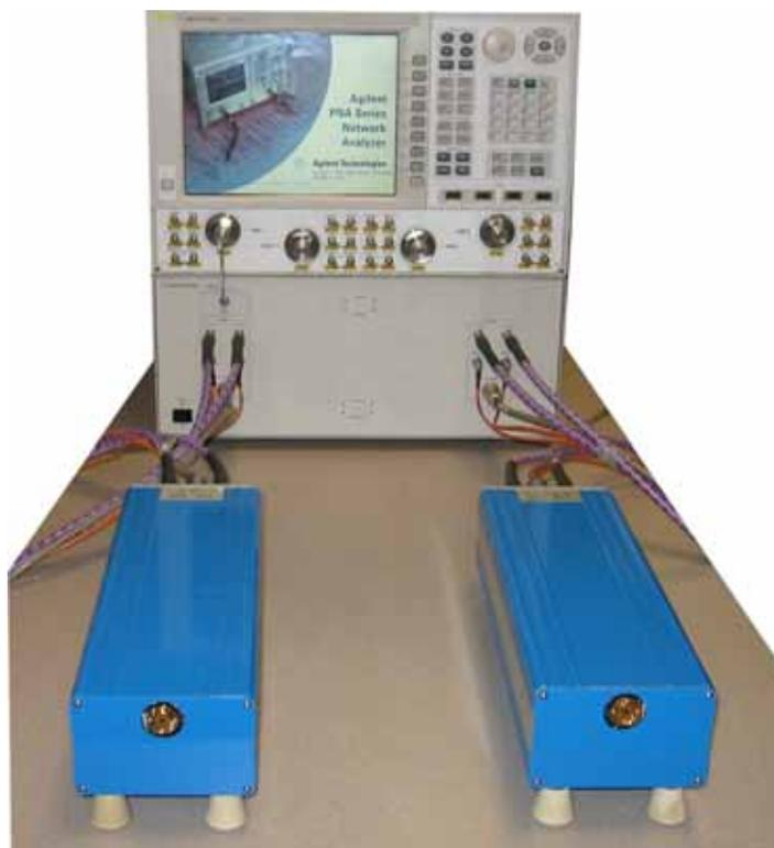
Figure 1-2 4-Port Banded Millimeter-wave Configuration (N5262A)
