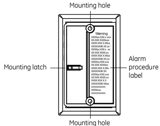
Figure 6: Horizontal mounting
