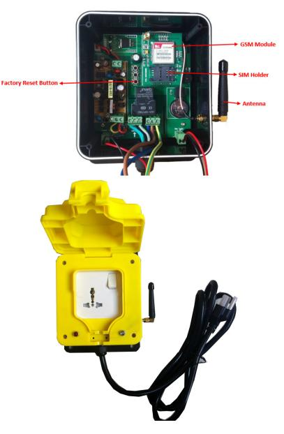
Insert the SIM card, to access the SIM card holder gently push the button adjacent to it, insert the SIM card and carefully close the holder.
