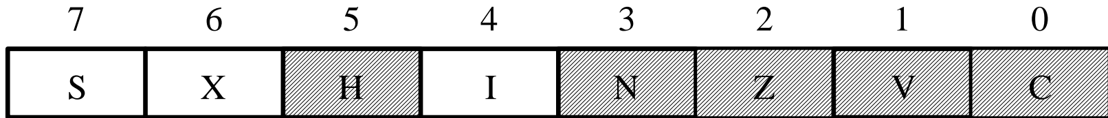
Figure 2.8 Condition code register
