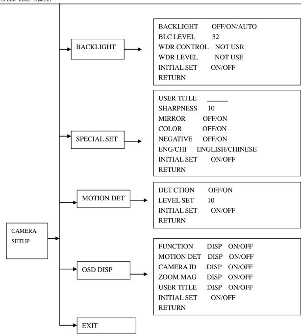
Remark: LG zoom module , use the keyboard to enter to the menu , the "FOCUS+" and "FOCUS- can change the parameter , "ZOOM+" and "ZOOM-" can change the cursor position .
