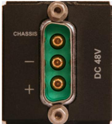
Figure 2: The CHASSIS-1- DC Power Plug
