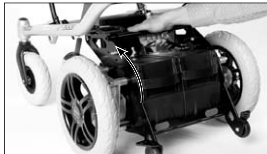
Fig. 10 Securing the battery packs
