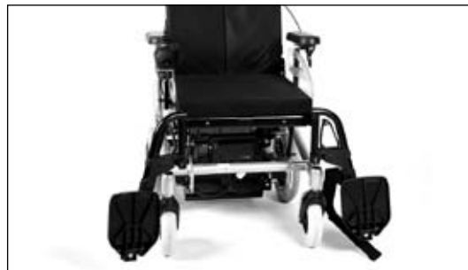
Fig. 19 Footrests swung to the side
