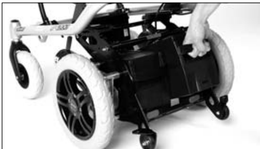
Fig. 23 Removing battery pack
