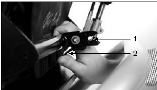
Fig. 26 Cross bolt locked in the holding device
