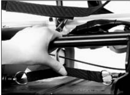
Fig. 6 Seat lock release
