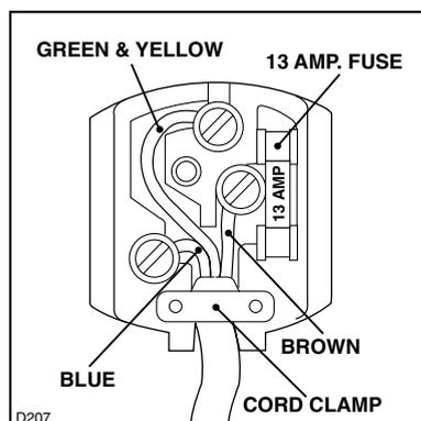
Connect the Green and Yellow (earth) wire to the terminal in the plug which is marked with the letter «E» or the earth symbol
