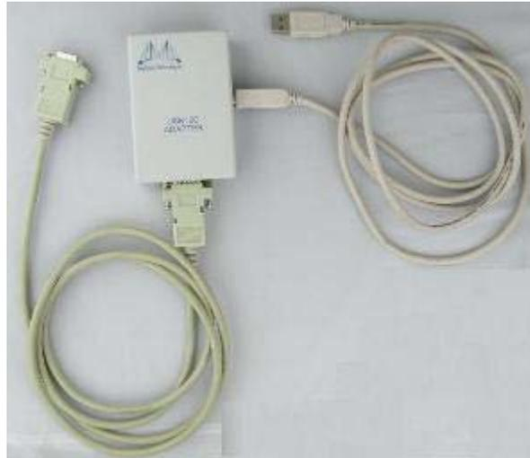
The MTUSB adapter comes with three cables, but has only two connections for cables. One cable is an I2C cable with DB9 female connectors on both ends. One cable is a I2C cable with DB9 female connector to RJ45 male. Use the cable that matches your switch. The other is a USB cable with one type A host connection to be connected to the server or PC and a type B connection to be connected to the MTUSB adapter.
