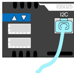
With the switch connected to a computer through the MTUSB, it is now possible to reprogram the SPI Flash memory.
