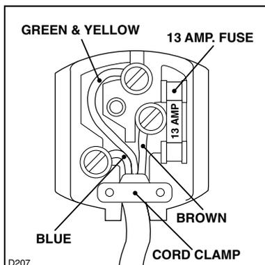
Connect the Green and Yellow (earth) wire to the terminal in the plug which is marked with the letter «E» or the earth symbol
