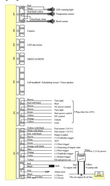
\*Orange with black wire of JP1: Engine status detection, it is used to detect the engine started or not after automatically start command, this wire connects to the power wire of fuel pump(for gasoline vehicle) or output wire of generator (for diesel vehicle), and it has 9V-14V voltage after engine started.
