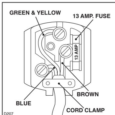
Connect the Green and Yellow (earth) wire to the terminal in the plug which is marked with the letter «E» or the earth symbol
