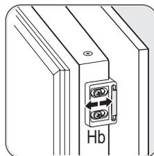
Place the small square on the guide again and fix it with the screws supplied. Align the kitchen furniture door and the appliance door by adjusting the part Hb.
