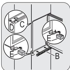
Attach the covers (C, D) to the lugs and the hinge holes.
