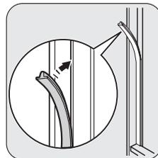
Push the sealing strip between the appliance and the adjacent cabinet.
