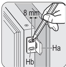
Open the appliance door and the kitchen furniture door at an angle of 90°. Insert the small square (Hb) into guide (Ha). Put together the appliance door and the furniture door and mark the holes.
