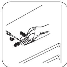
lamp of the same power and specifically designed for household appliances (the maximum power is shown on the lamp cover).
