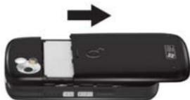
2. Hook and lift the battery upward as shown below in order to remove it.
